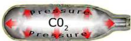
For all the dragsters in the challenge, a CO<sub>2</sub> charger provides the force to move the vehicle forward. The chargers contain a large volume of carbon dioxide gas under extreme pressure. The firing pin on the start gate makes a hole in the nozzle so the pressurized CO<sub>2</sub> gas escapes producing thrust or force.
